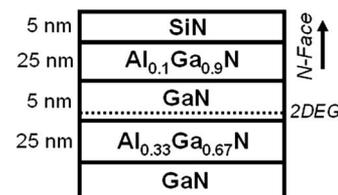
FIG. 1. Epitaxial structure of the N-polar HEMT used for both theoretical calculations and experimental measurements in this study.
