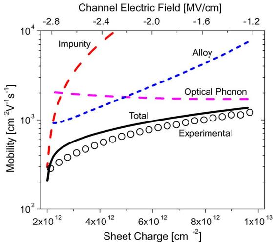
FIG. 3. (Color online) Theoretical calculations for mobility limited by optical phonon, ionized impurity and alloy disorder scattering, the total mobility, and the experimentally measured data plotted vs 2DEG sheet charge and channel electric field as the gate is pinched off.
