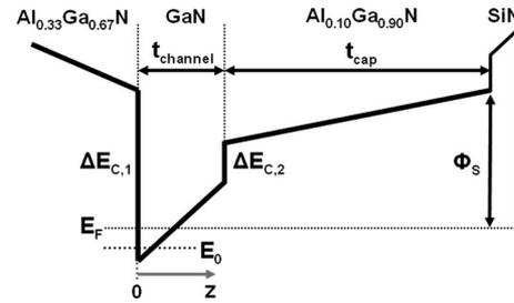
FIG. 2. Conduction band diagram of the HEMT used in this experiment. The N-polar surface is on the right hand side.
